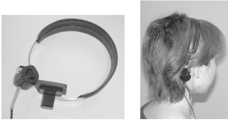
Figure 2: Ceramic vibrator of the BCUHA attached to the mastoid with a hair-band-like device
