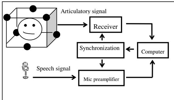
Figure 2: Schematic diagram of EMA setup
