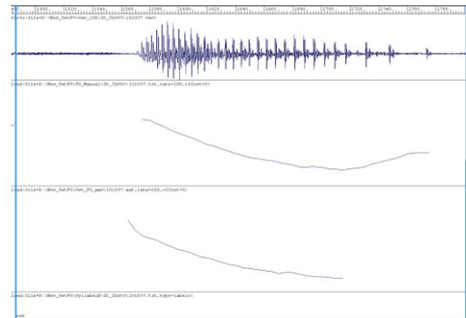
Figure 3: An example of  $F_0$  contours of Mandarin syllable "sa4". From top to bottom: original wave,  $F_0$  by manually check,  $F_0$  calculated by RAPT algorithm.
