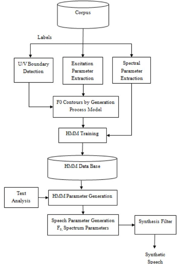
Figure 5: A HMM-based TTS with Generation Process Model and  $VU$  decision
