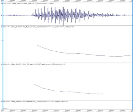
Figure 4: An example of  $F_0$  contours of Mandarin syllable “zou3”. From top to bottom: original wave,  $F_0$  by manually check,  $F_0$  calculated by RAPT algorithm.
